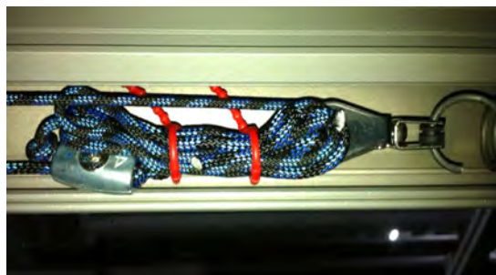
Tensioning rope fixed with cable ties
