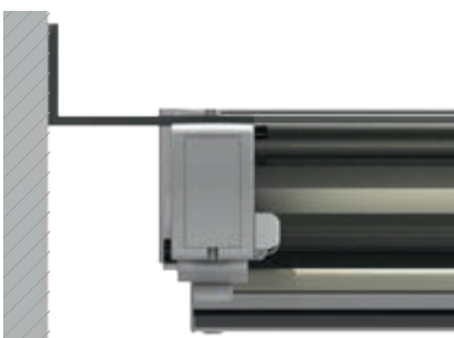
Installation of the weinor PergoTex II Basic in a niche or laterally on a wall using the 200 x 100 x 10 x 120 mm angle bracket
