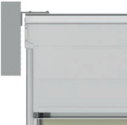
Installation laterally on a wall or in a niche using the 200 x 100 x 10 x 140 mm angle bracket
